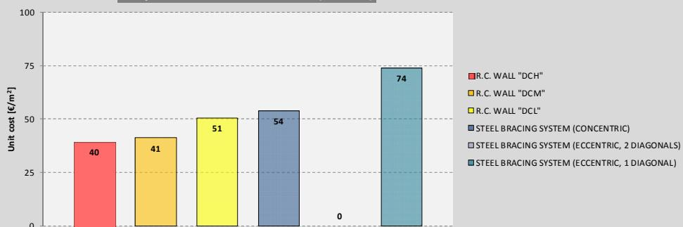
**COMPARISON BETWEEN R.C. WALL AND STEEL BRACING SYSTEMS (B=8m; H=8m; V<sub>b</sub>=1500 kN)**
