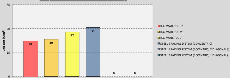
**COMPARISON BETWEEN R.C. WALL AND STEEL BRACING SYSTEMS (B=8m; H=8m; V<sub>b</sub>=2000 kN)**
