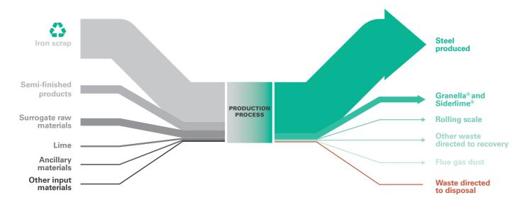
Qualitative representation of the flow of materials into and out of the production process of the 3 meltshops of the Group.
