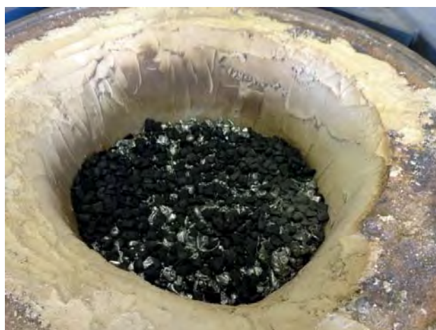
Figure 49. Crucible of pilot furnace charged with a first scrap layer and biochar briquettes (BCB)
