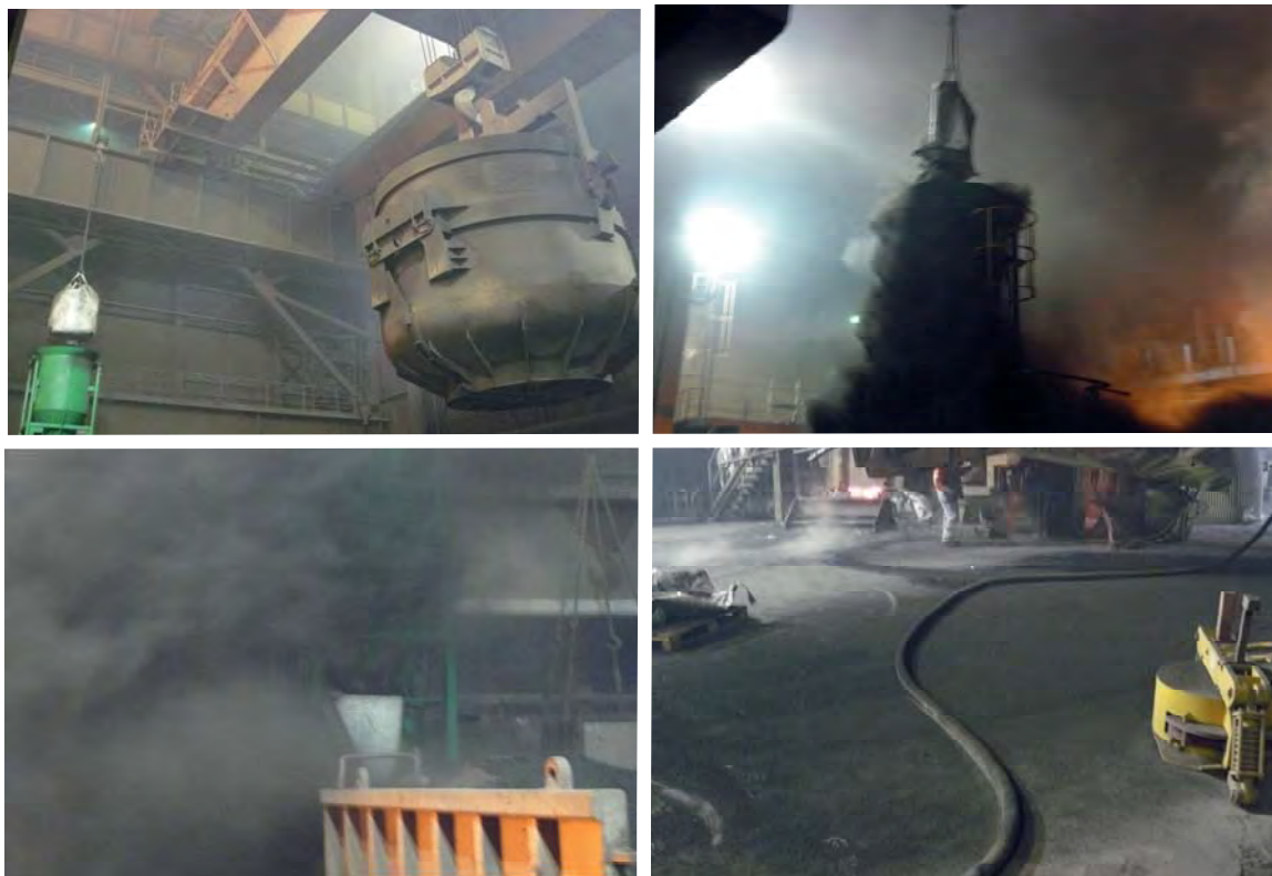
Figure 65. Problems occurring while using biochar fines as injection coal
