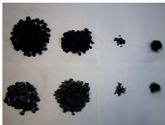
Figure 48. Grain size distributions (left) and mass fractions (right) after drop tests
