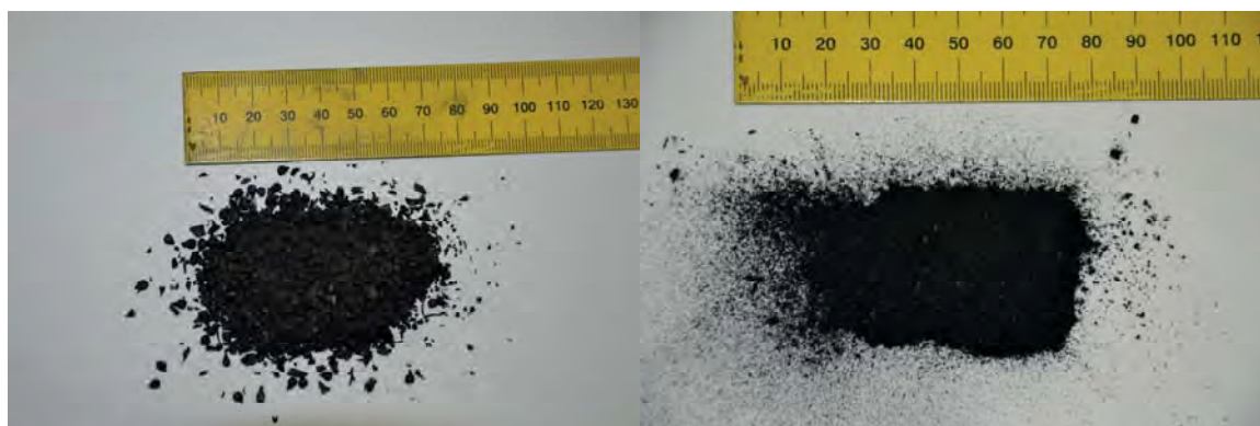
Figure 38 Biochar from Tecnocentro (left); Biochar from wood gasification plants (right)
