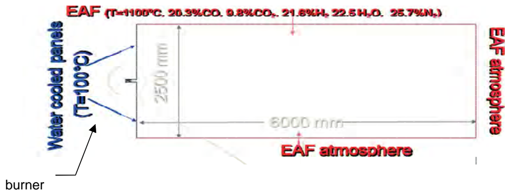
Figure 72. Boundary conditions used for CFD calculations
