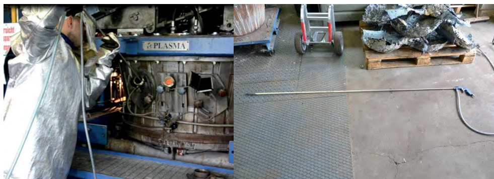
Figure 41. Lancing operation of coal and oxygen (left) and IOB pilot lancing system (right)
