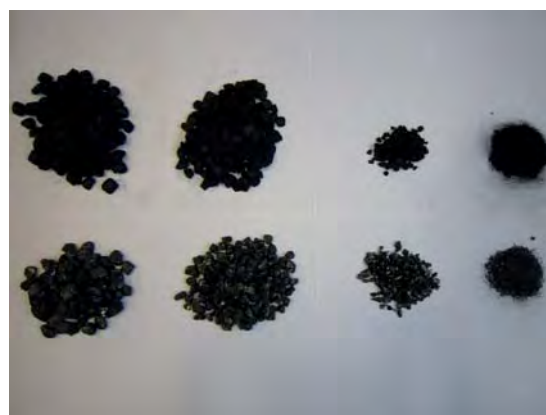
Figure 47. Grain size distributions (left) and mass fractions (right) after vibrating sieve tests
