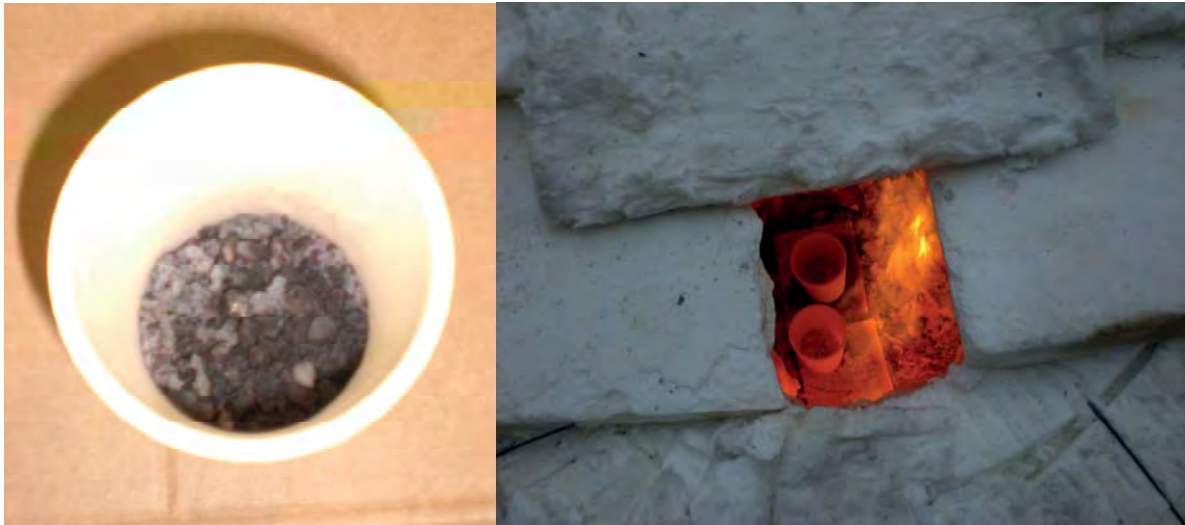
Figure 31: Crucible filled with slag and carbon mixture (left) and crucibles in the furnace (right) in lab experiment carried out by RWTH.
