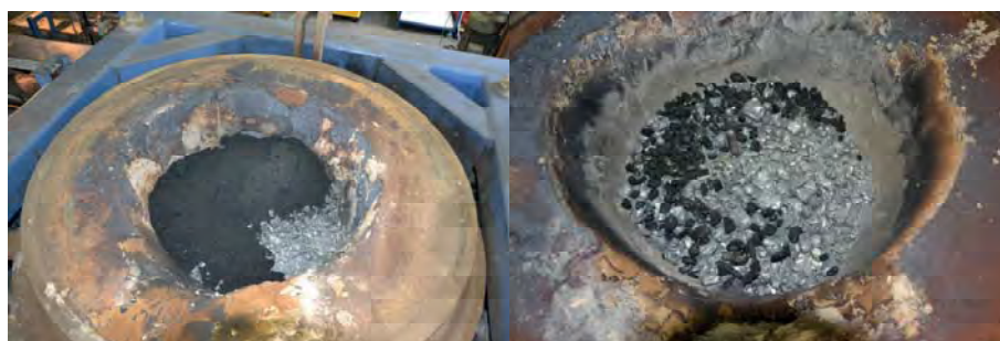
Figure 40. 1.6 kg of biochar fines (left) and 1 kg of anthracite coal (right)
