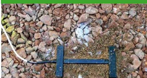
Figure 4.2a Placing of the sensors in the subgrade
