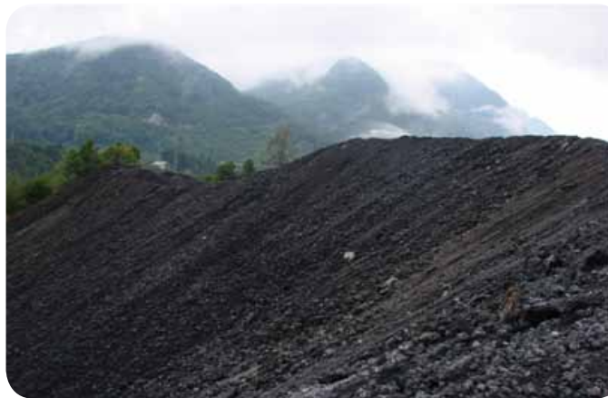
Aggening of slag for 30 days
