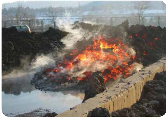
Quenching of hot slag
